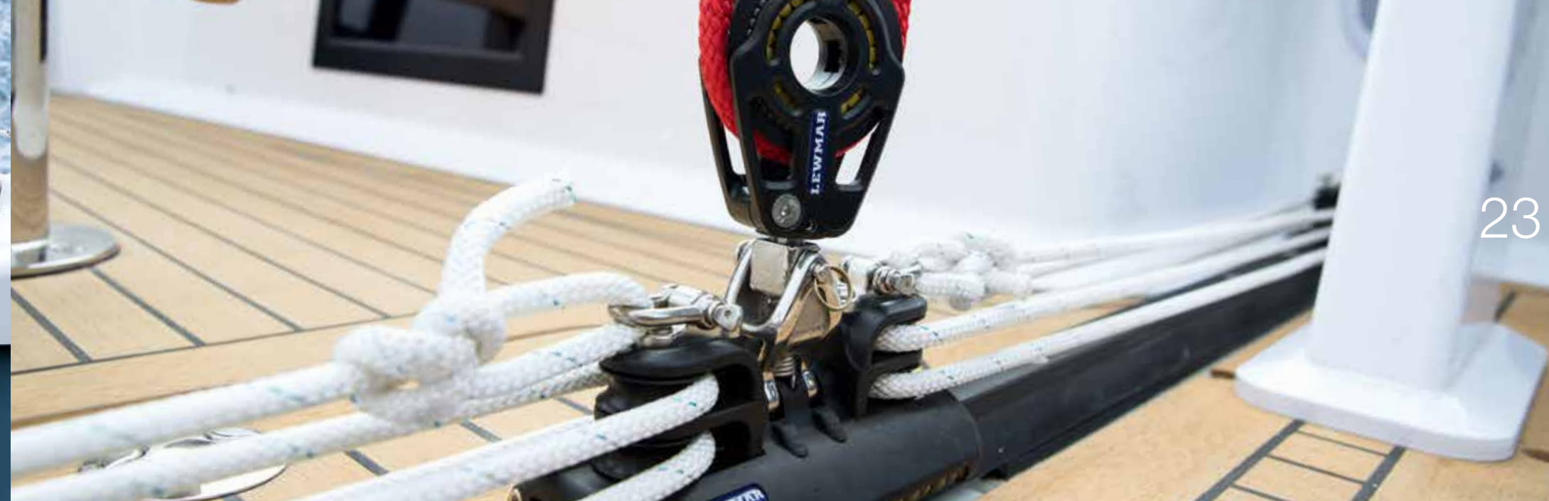
Recessed into the floor, the mainsheet traveller allows an ideal trim of the mainsail.
