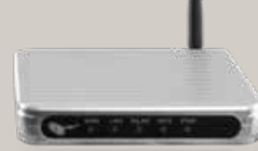
WLAN access point
