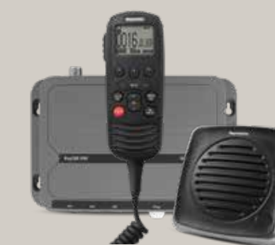
Raymarine 260 VHF at chart table incl. 2nd wireless handset
