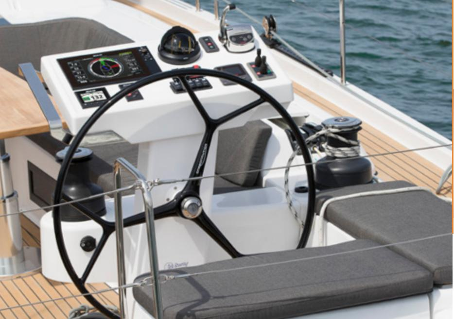
2 instrument pods | B&G Autopilot with 2 Triton<sup>2</sup> control units and precision 9 compass
